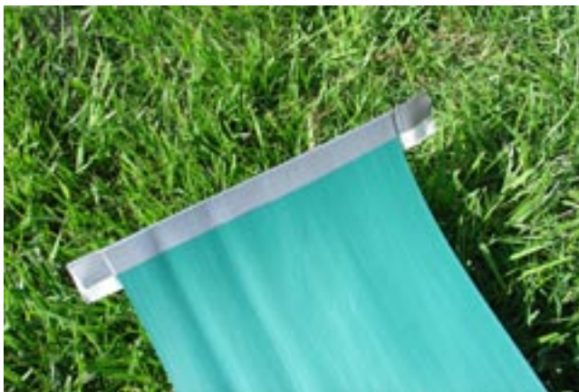
Tape/Cement the end of the belt that is not inserted into the collection pipe.
